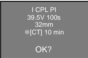
**Note:** In case of barcode scanner failure you can still set the welding parameters manually (below). Press OK ► to proceed.
