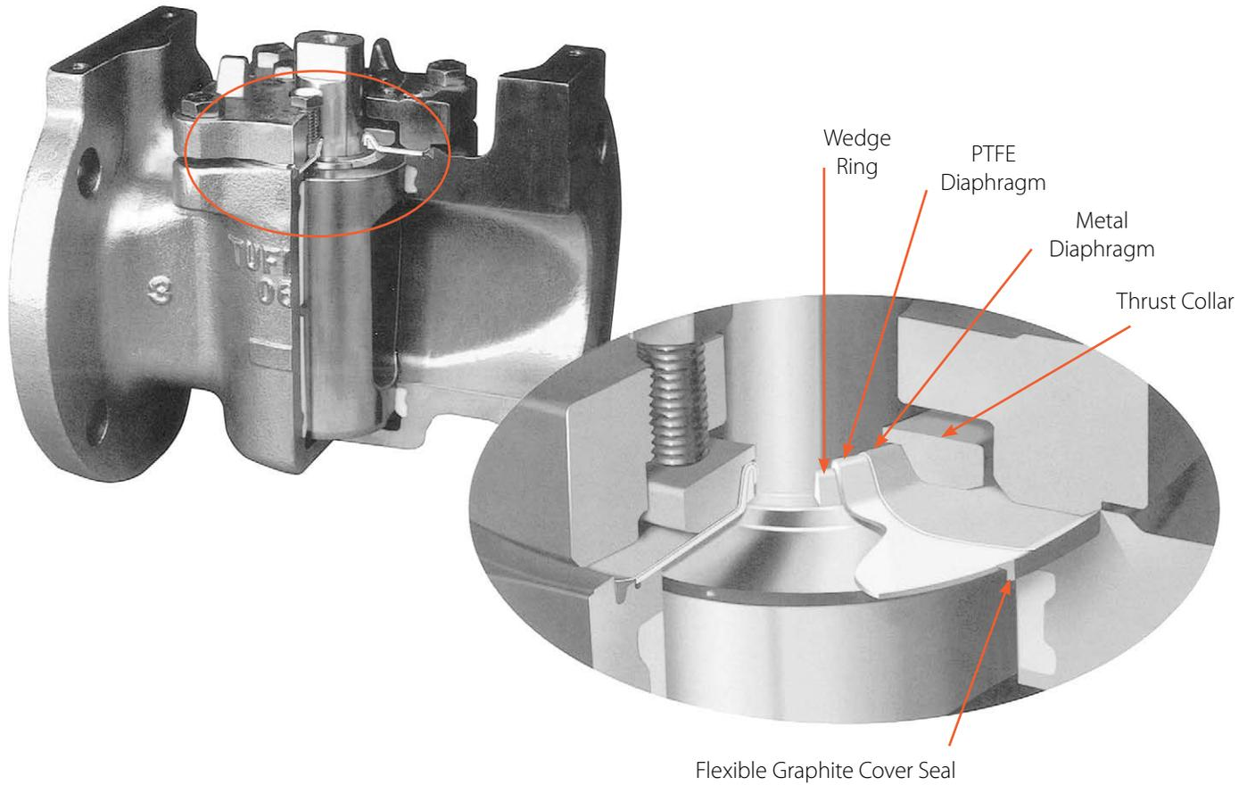
Tuflin Fire-Tested Sleeved Plug Valves have been tested in accordance with API-607 - Fourth Edition - Section 4.2 - Specifications For External Leakage. These valves exceed the sealing requirements specified in those standards. A tight external seal was maintained even after the PTFE sleeve and sealing parts were totally destroyed by fire.
